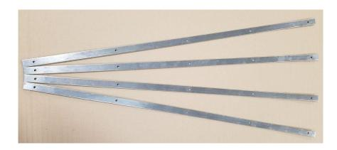
The Aluminum Batten Strips are required for use with the ENPAC Drive-Over Diverter Berm. They are applied on top of the edges of the Diverter Berm and combined with a sealant to anchor the berm to the floor. Batten strips come with pre-drilled, 1/4" holes and are 4' in length for efficient shipping and easy handling.
